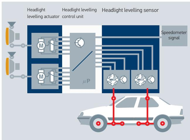
Circuit diagram of dynamic headlight range adjustment
