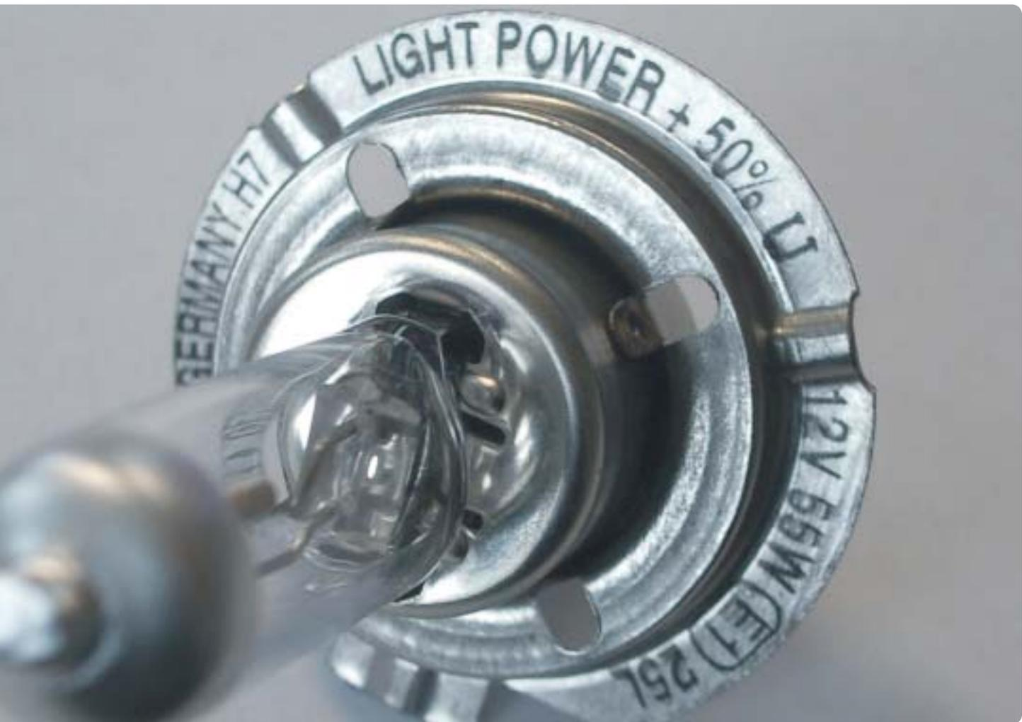
Vehicle bulbs have to be standardised in compliance with ECE-R37 or R99. This makes bulb replacement possible while at the same time avoiding mix-ups with other bulbs.
