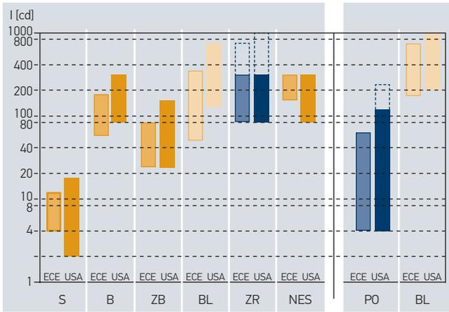
The permissible light intensity values are different depending on the function involved. Lights indicating changes in movement (brakes = 60 cd) radiate stronger light signals than those for position and orientation (taillight = 4 cd).
