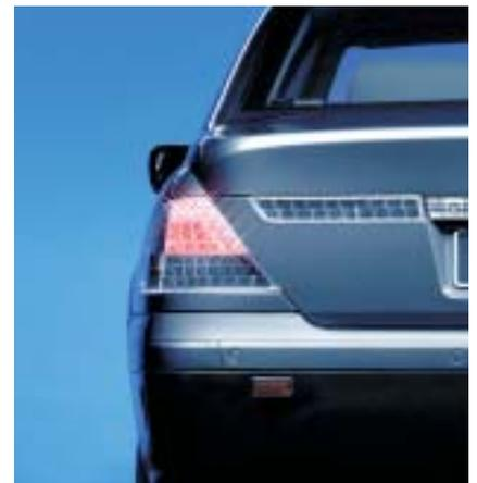
All the functions in a rearlight only work on one brightness level, no matter whether they are switched on during the day, at night or on a bright foggy morning. The only current possibility of adapting the lights to adverse weather conditions is the rear fog light. This is often used incorrectly, however, and leads to irritation. There is no additional information conveyed about whether the brakes are only being applied lightly or slammed on, for example.
