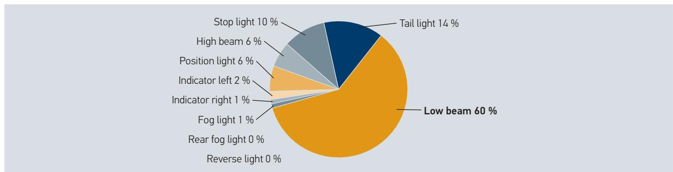
The above graphic represents 100 % of the energy requirements of a vehicle that is equipped with a combination of incandescent lamps (rear lights) and Halogen lamps (headlights). It is easy to see the greatest consumer of electrical energy. 60 % of the required energy are needs just for the low beam.
