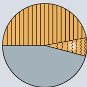
D Typical low beam distribution on the lens of a paraboloid headlight
