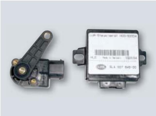
Headlight range adjustment sensor and control unit
