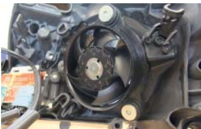
In order to improve cooling further, the air circulation is raised by axial or radial blowers between the cooling elements. Here is the axial blower in the Audi A8.
