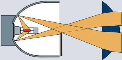
**B** Generation of the cut-off and slight shuttering by the shield (side view)
