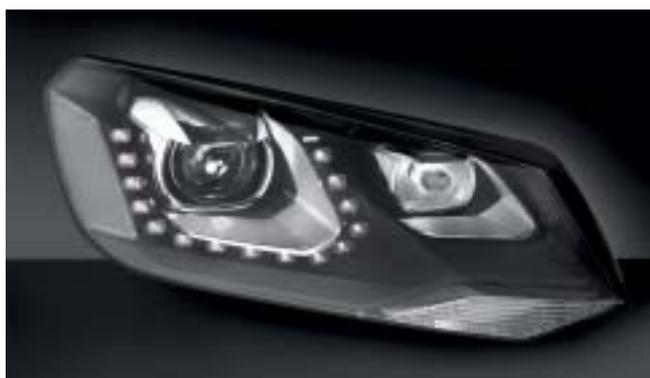
A glare-free high beam is offered, for instance in the VW Touareg.
