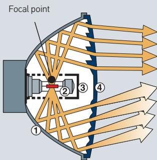
C Light deflection through prisms and light scatter through cylindrical patterns in the lens (seen from above). Useful light approx. 27 %.
