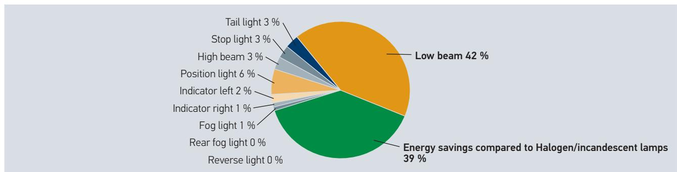
Just using a combination of Xenon lights and LEDs allowed the energy consumption to be lowered by 39 %.
