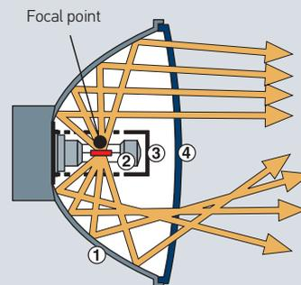
**C** Deflection and scatter of the light directly by the reflector surface. Useful light approx. 45 %.
