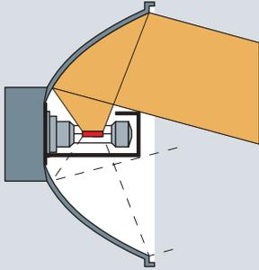
B Reflection of the light onto the road, seen from the side
