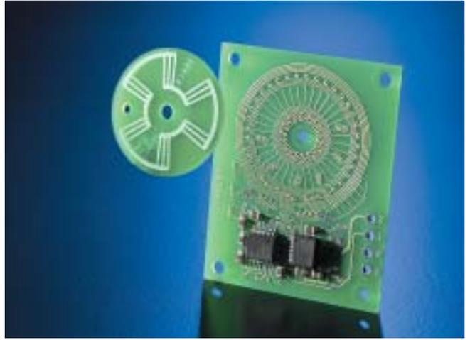
**Sensor-integrated headlight range adjustment control unit**
