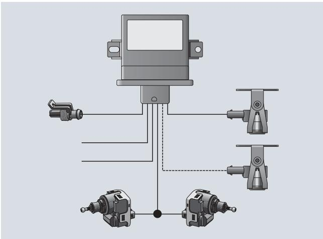
Central control unit for ultrasound headlight range adjustment
