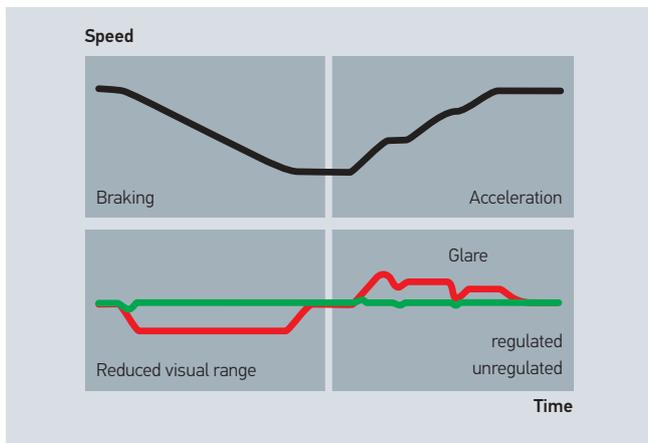
Headlights with and without dynamic headlight range adjustment during braking and acceleration
