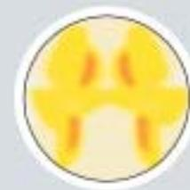
**D** Example of light distribution on the cover lens of an FF headlight
