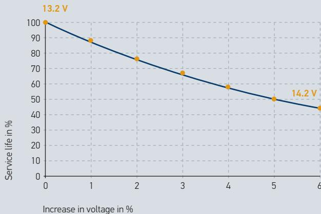
For this reason dropping resistors are used in some vehicle types to prevent the supply voltage exceeding 13.2 V. In today's modern vehicles, the voltage is adjusted through pulse-width modulation. In the case of undervoltage, e.g. if the alternator is faulty, the opposite is the case. The light now has a significantly higher red share and the light output is correspondingly lower.
